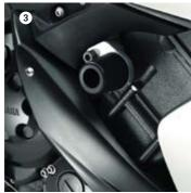
Roller Protector YEC engineered. Anodized T6 aluminium brackets and high impact Nylon rollers. 5VY-W0741-00-00
